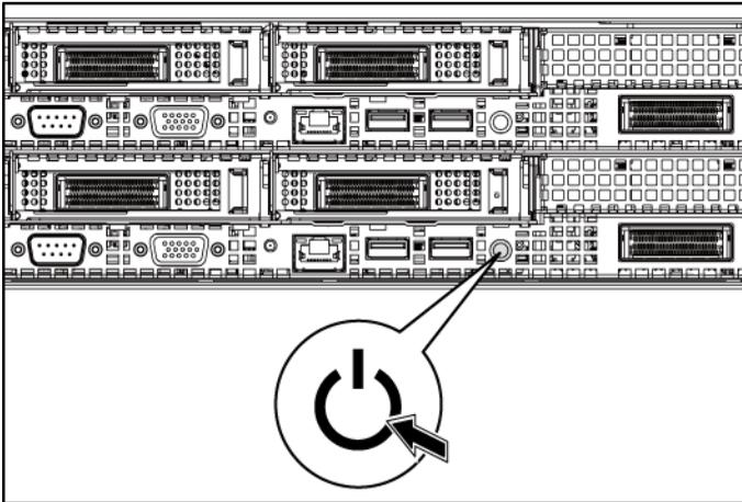
Press the power button(s) either on the front or back of the system and on the monitor. The power indicators should light.
